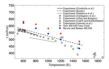
FIG. 7. A comparison of the predicted vapor-liquid surface tensions for the two MEAM force fields with experimental data. Experimental data are taken from Friedrichs *et al.* [76], Keene [77], Dalakova *et al.* [63], Alchagirov *et al.* [78], Allen and Kingery [79], Cahill and Kirshenbaum [80], and Gancarz *et al.* [64]. Error bars for simulation results, representing the 95% confidence interval, are smaller than the symbol size.
