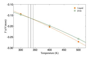
FIG. 1. Helmholtz free energy at zero pressure for the  $\beta$ -tin crystal and liquid tin using the Ravelo and Baskes force field. Error bars for free energy, representing the 95% confidence intervals, are smaller than the symbol size. Orange and green solid lines are fits to the data points. The black solid line represents the melting point and the black dotted lines represent the 95% confidence interval.
