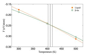
FIG. 2. Helmholtz free energy at zero pressure for the  $\beta$ -tin crystal and liquid tin using the new MEAM force field. Error bars for free energy, representing the 95% confidence intervals, are smaller than the symbol size. Orange and green solid lines are fits to the data points. The black solid line represents the melting point and the black dotted lines represent the 95% confidence interval.
