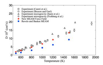
FIG. 5. A comparison of the predicted self-diffusion coefficients for the two MEAM force fields with experimental data. Experimental data are taken from Careri *et al.* [65], Bruson and Gerl [39], Itami *et al.* [66], and Frohberg *et al.* [67]. Error bars for simulation results, representing the 95% confidence interval, are smaller than the symbol size.
