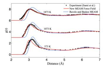
FIG. 3. A comparison of the predicted radial distribution functions g(r) for the two MEAM force fields with experimental data. Experimental data are taken from Itami *et al.* [25]. The radial distribution functions at higher temperatures have been vertically shifted for clarity.
