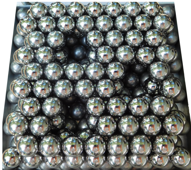
FIG. 9. Photograph of a mechanically stable ball-bearing arrangement in two adjacent layers of three nearest-neighbor trivacancy tunnels.
