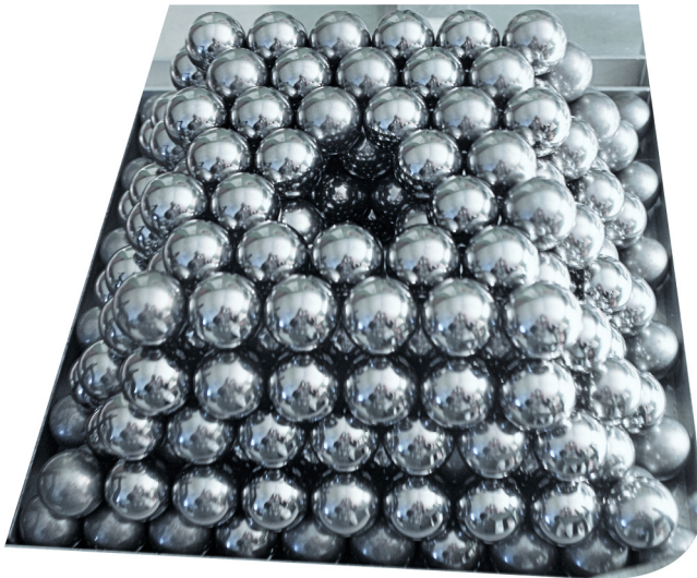
FIG. 6. Photograph of a ball-bearing stacking ( N = 336 ) with four layers of a single trivacancy tunnel. Each ball bearing has a diameter of 11/16 in.
